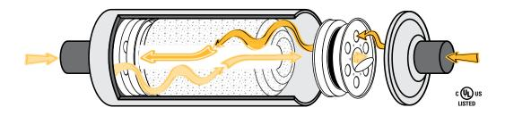
The BF Series bi-flow filter-drier is designed specifically for heat pump or a reverse cycle application. External check valves are not required since they are incorporated within the filter-drier.
