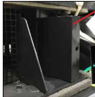
*Reversible fresh air filter provides 23 cfm of fresh air exchange.*
