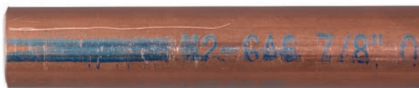
Figure 2 - Copper tube with “bad” surface scratch.
