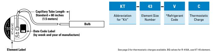
Selecting The Cartridge — See table on previous page for cartridge codes.Q Valve Cartridge Service Kit — Part No. 184000BQ Valve Cartridge Service Kit — Part No. 184007
