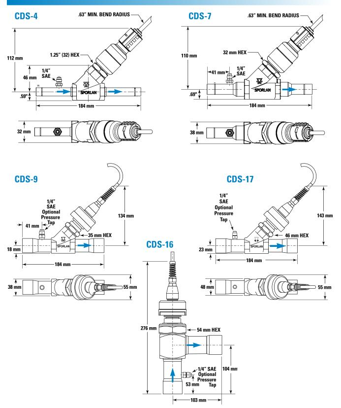
**CDS** – **Valve Nomenclature/Ordering Instructions** The CDS-16 is the only angled valve. The CDS-4, CDS-7, CDS-9 and CDS-17 are straight through valves.
