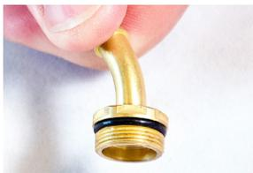
Install the barb seal o-ring by gently stretching and pulling it over the threads of the barb fitting. Place the barb seal in the groove located between the hex feature and the back portion of thread ensuring the seal is not torn or damaged.
