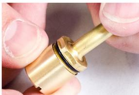
Screw cup assembly with spring onto hose barb fitting. Hold cup so that the spring is in an upward position while screwing onto the hose barb. This ensures that the spring remains properly seated. Hand tighten the cup to the barb ensuring cup seats over the barb gasket (o-ring) and does not damage the o-ring.
