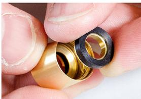
Insert bushing/seal into the thread side of the cup. Brass bushing side goes in first with seal facing up as shown.
