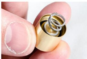
Place spring into cup assembly over the boss on the back side of the depressor.
