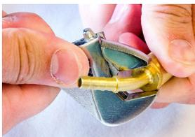
Tighten the cup and hose barb using the 9/16" open end wrench and 1/16" steel blade. Do not over tighten. Only 25 to 30 in/lbs is required.
