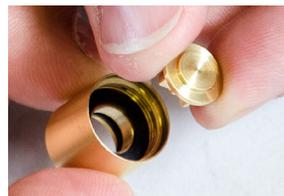
Insert depressor with 3 blade feature into the cup assembly. The depressor fits into the bushing/seal installed in the previous step. The depressor must sit flat and true to the seal surface.
