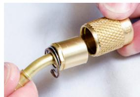
Insert barb/cup assembly into the coupler. Place thrust washer into coupler such that the thrust washer is seated flat onto the hose barb and inside the Coupler. Now install the internal snap ring. Ensure the snap ring is seated properly into the groove of the coupler. This completes the rebuilding process.
