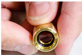
Hold the cup in one hand so that the slotted face of the cup is exposed. Pinch the cup seal o-ring and insert it into the large groove to seat it correctly as shown.
